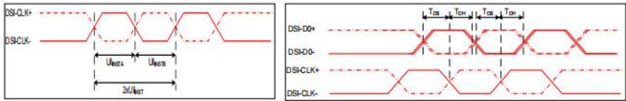
Figure 4 DSI clock channel timing
