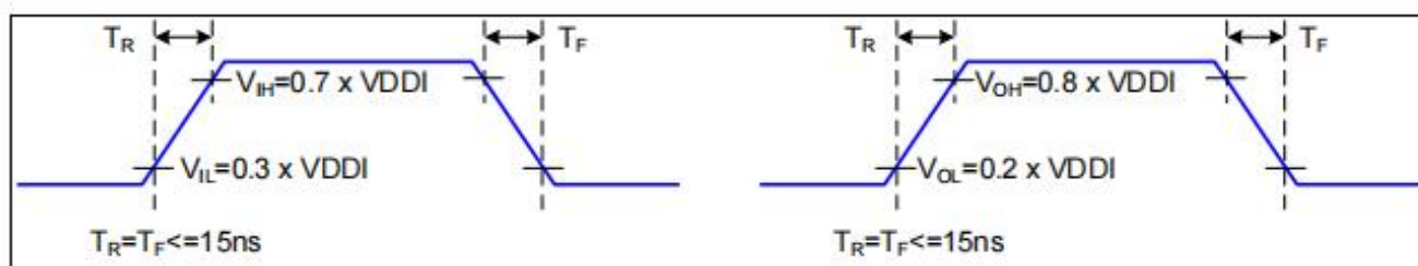
Figure 2 Rising and Falling Timing for I/O Signal
