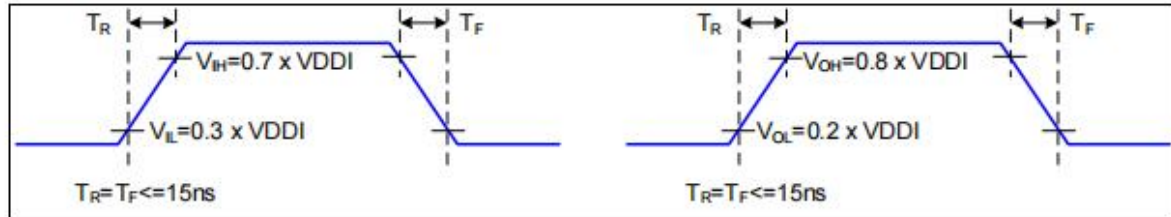
Figure 2 Rising and Falling Timing for I/O Signal
